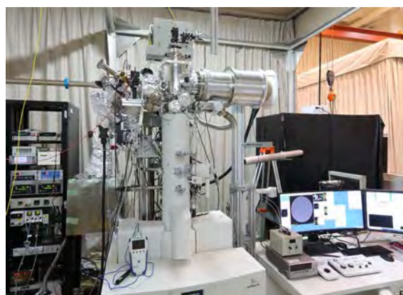
Figure 1. The newly developed 100 kV TRTEM system based on an HT7830 (Hitachi High-Tech Corp.).
